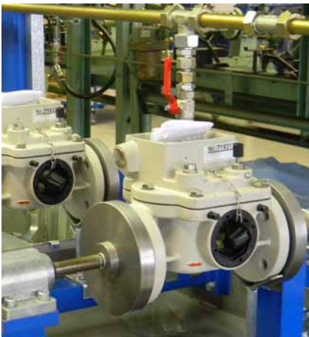
Figure 4.1. - Functional and leakage test
